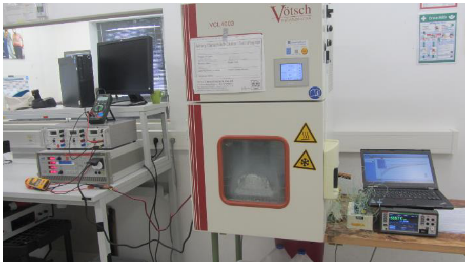
Figure 17: Sample A during Continuous Device Operation to Determine External Surface Temperatures
