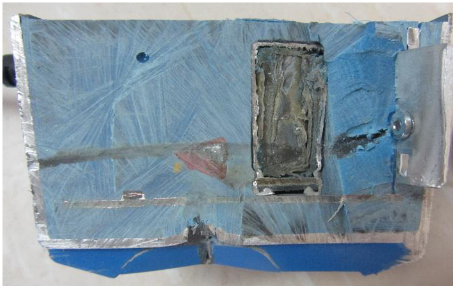
Figure 25: Part of Sample E opened after Method of Test—Sealed Devices
