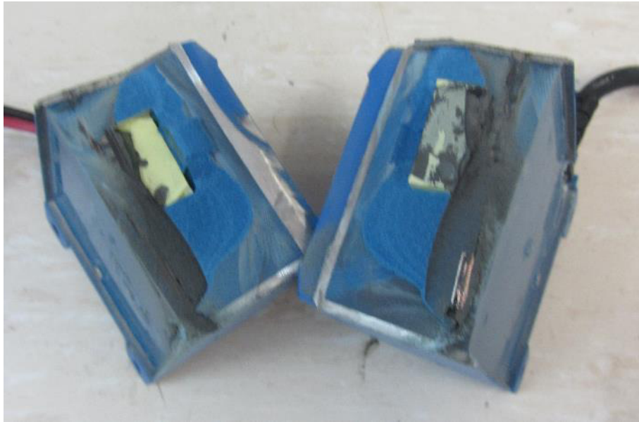
Figure 24: Parts of Sample C opened after Method of Test—Sealed Devices
