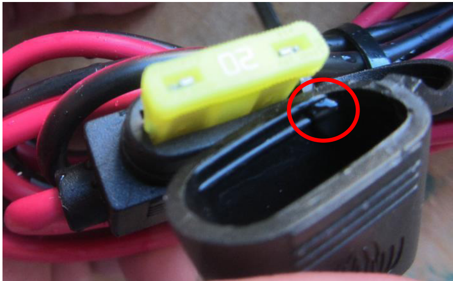
Figure 22: Detailed view of water drop in the fuse box of Sample B after Method of Test—Sealed Devices
