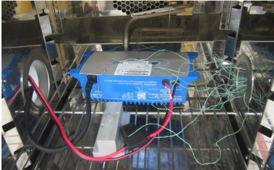
Figure 18: Sample D during Continuous Device Operation to Determine External Surface Temperatures – inside climate chamber
